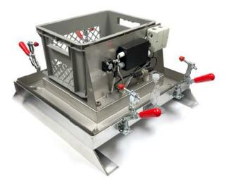
Rear of CūrPod mini showing Sensor Array
